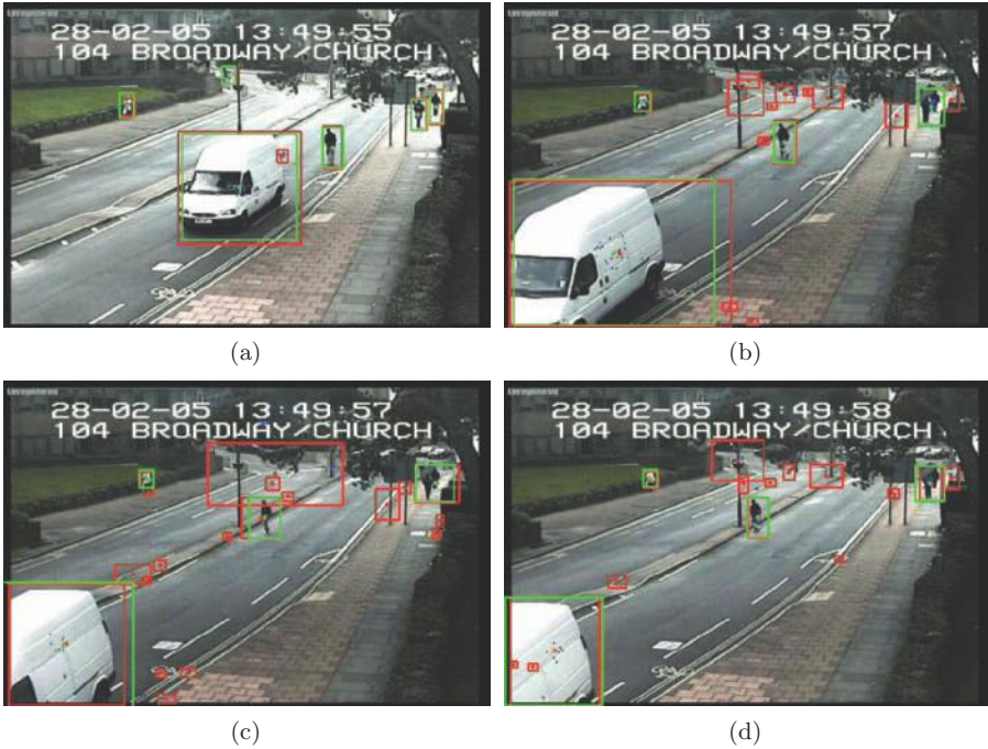
Figure 7.8 Comparison of tracking results on an outdoor surveillance scenario between raw object detections (colour-coded in red) from a background subtraction module and PHD filter output (colour-coded in green). Several false detections are filtered by the PHD (b, c, d). IEEE © [33].
