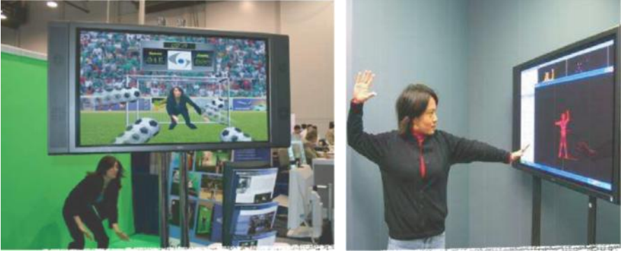
Figure 2.10 Examples of gesture interfaces for interactive gaming. The video camera uses tracking technology to capture the gestures that are converted into gaming actions. Reproduced with permission of GestureTek.
