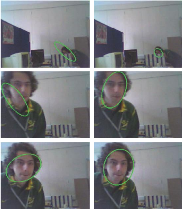
Figure A.3 Sample tracking results for the test sequence H6 (frames 715, 819, and 864) using different target representations: HY-OH (left) and HY-SH (right). Reproduced with permission of Elsevier [1].
